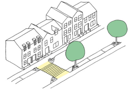
Figure 36: A sketch highlighting pedestrian crossings and on street trees - inclusion of these features can also help to reduce traffic speeds.
