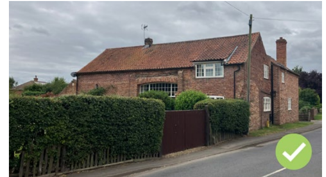
Figure 16: Clusters of old farm buildings with L-shaped arrangements are common, with main facades rotated at 90 degrees to the street, creating courtyards. Often gable ends extend right up to the pavement with no setbacks.
