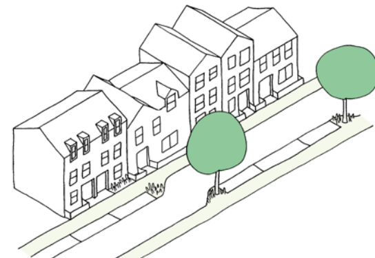
Figure 37: A sketch showing a road with on-street parking and chicanes. New development should consider integrating traffic calming measures such as these to help reduce traffic speeds without the need for speed bumps.
